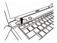
Figure 4-12 Removing the keyboard cover
